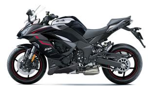
Dual 300mm discs with radial-mount 4-piston
